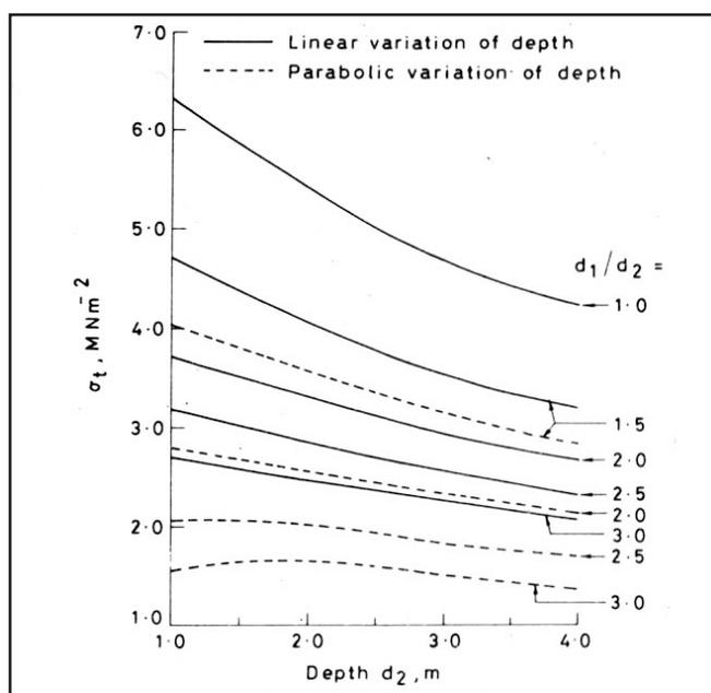
Figure 10. Variation of soffit stresses at the intermediate support section of two-span continuous non-prismatic T-beams
