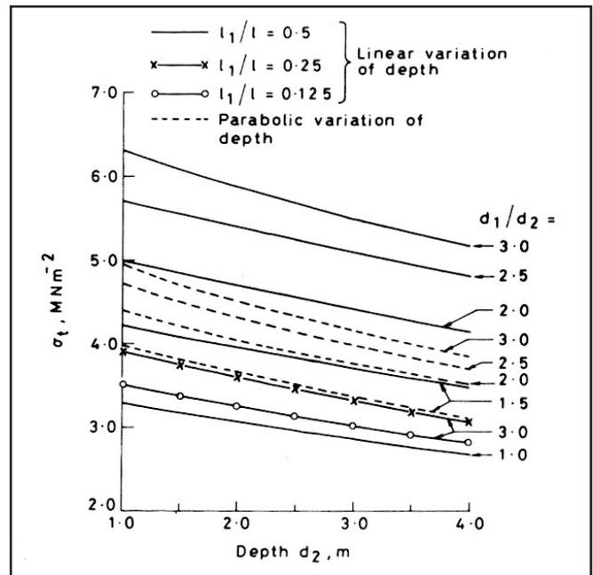
Figure 8. Variation of mid-span soffit stresses in multi-span continuous non-prismatic box girders
