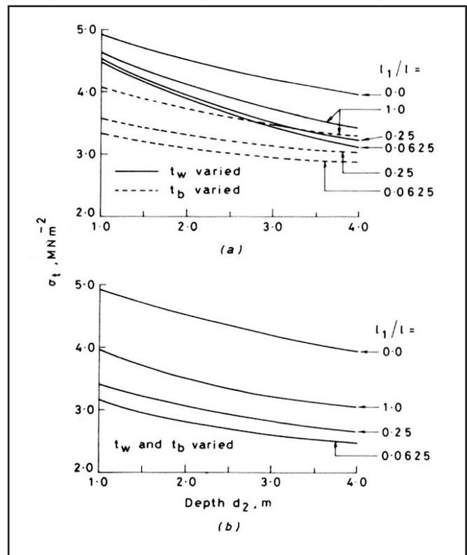
Figure 14. Variation of soffit stresses at the intermediate support section of two-span continuous non-prismatic box girders of constant depth
