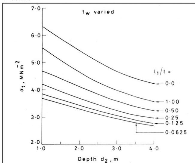
Figure 11. Variation of soffit stresses at the intermediate support section of two-span continuous non-prismatic T-beams of constant depth
