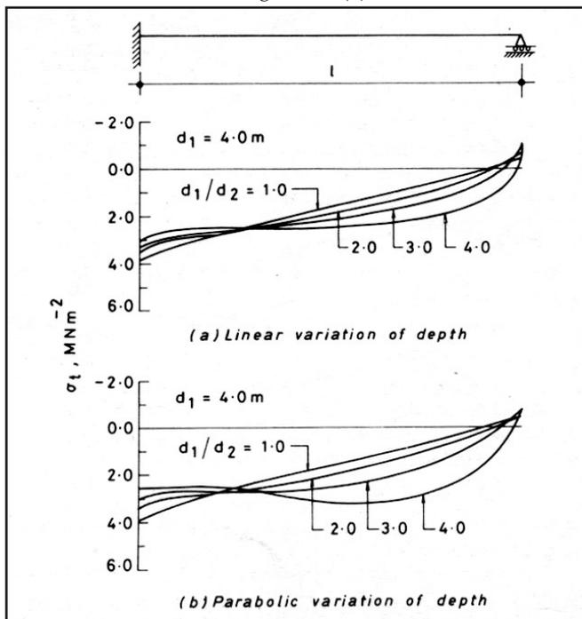
Figure 15. Variation of soffit stresses along the span in two-span continuous non-prismatic box girders
