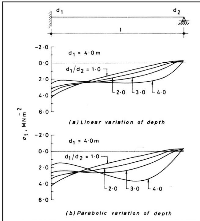
Figure 12. Variation of soffit stresses along the span in two-span continuous non-prismatic T-beams
