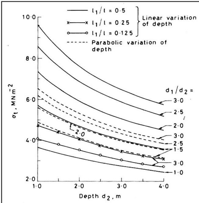
Figure 6. Variation of mid-span soffit stresses in multi-span continuous non-prismatic T-beams
