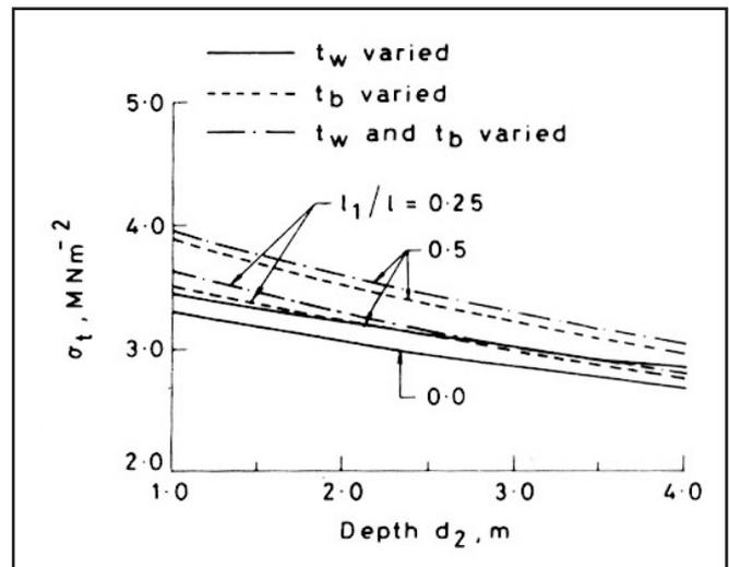
Figure 9. Variation of mid-span soffit stresses in multi-span continuous non-prismatic box girders of constant depth
