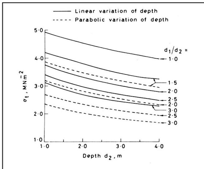
Figure 13. Variation of soffit stresses at the intermediate support section of two-span continuous non-prismatic box girders
