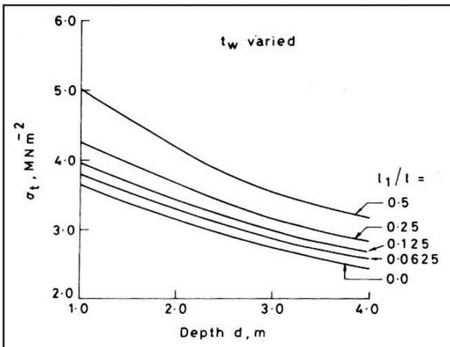
Figure 7. Variation of mid-span soffit stresses in multi-span continuous non-prismatic T-beams of constant depth
